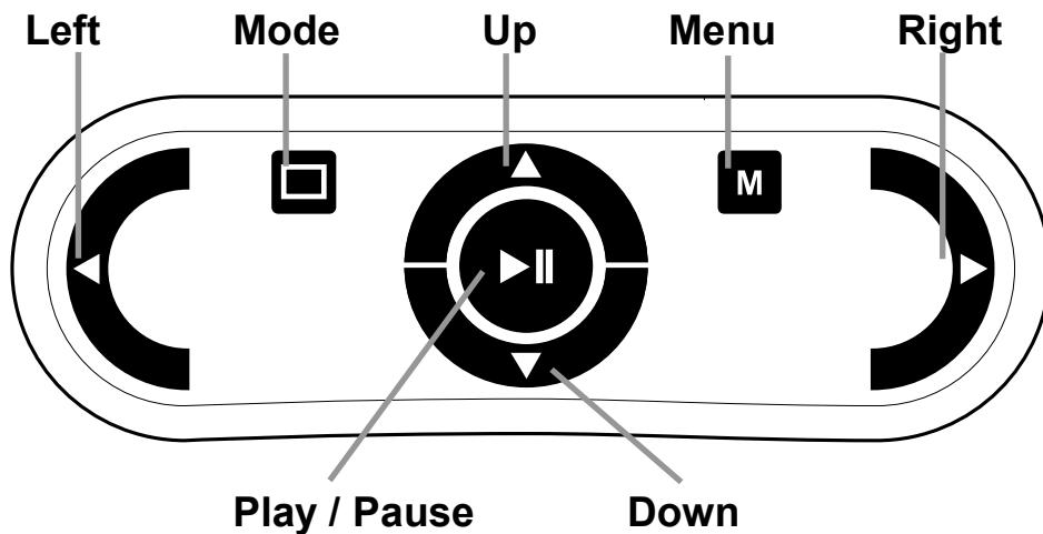
**Play / Pause button:** Round button in the centre of the remote control to stop and restart reading. Press and hold down the button for 2 seconds to spell the current word. Pressing the Play / Pause button within the menu will activate the button, cycle through the available options, check or uncheck the selection or enter a submenu.
